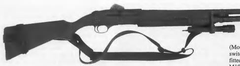
The Mossberg M9200A1 with all the refinements that bring it to the highest level as a fighting shotgun: Giles sling, MMC ghost ring sights, extended magazine tube, Vang Comp System and SURE-FIRE Tactical Light.
